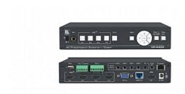
VP-440X is a high-performance 18G 4K HDR presentation switcher/scaler with four HDMI inputs and one computer graphics (VGA) input. It scales the video, embeds the audio, and outputs the signal to two identical outputs – one HDMI and one HDBaseT – together with an analog stereo audio output. Via HDBaseT, it extends video signals to up to 40m (130ft) over CAT copper cables at up to 4K@60Hz (4:2:0) 24bpp video resolution and provides even further reach for lower HD video resolutions
